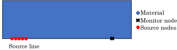
Figure 2.4: Schematic of the model used to improve the quality of Rayleigh waves in an FE model. This model contains a source line and a single monitor node.
