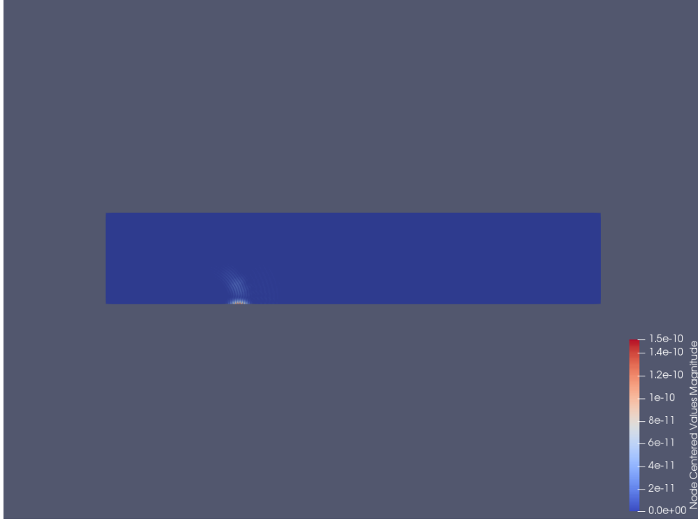
Figure 2.5: Rayleigh wave field, travelling in the positive x -direction created using the method described in this section. The colour scale in the figure represents the absolute magnitude of the displacement at each node. The Rayleigh wave's centre frequency is 10 MHz.
