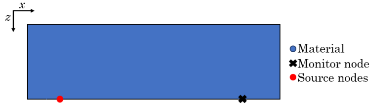
Figure 2.2: Schematic of the initial model used to derive the method for creating a good quality Rayleigh wave. This model contains a single source node and a single monitor node.
