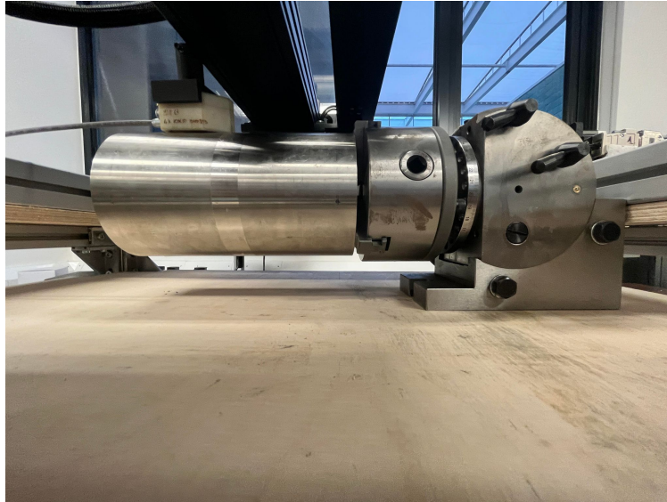
Figure 5.12: Setup used for obtaining a C_T C-scan of the area around the fatigue spots in the pipe shown. The EMAT, which is mounted on the scanning frame can move in the axial direction, while the pipe can be manually rotated using the indexing head each time the EMAT finishes the measurements on one line, to achieve a semi-automated C-scan.
