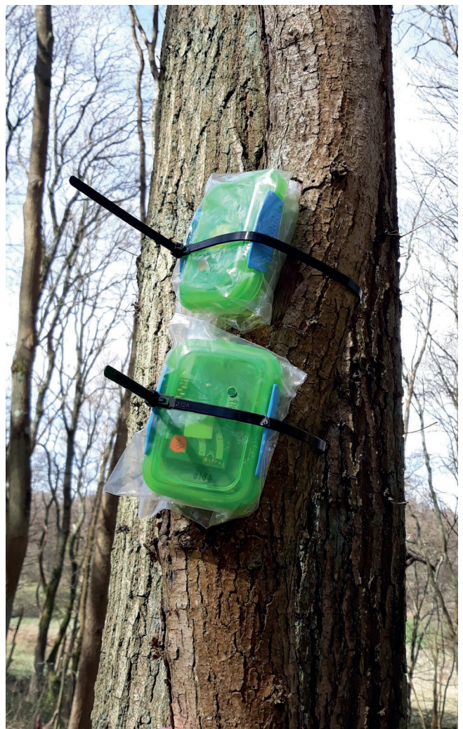
Audiomoths used to record bird and bat calls for biodiversity assessments (credit: C. Estrada)
