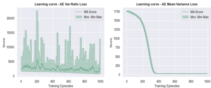
Figure B.5: Left: Learning curve of the linear AE with variance-ratio loss. Right: Same model with mean-variance loss
