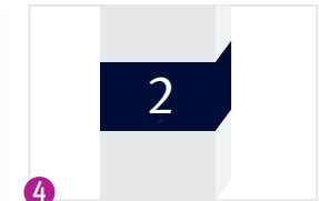
4 VC3 Lift Jamb Level Marker The Braille and tactile level number helps lift passengers to identify the current level.
